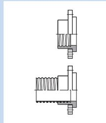
**Loose flange to fit mating flanges acc. to DIN 2632/2633, hole pattern DIN-EN 1092-1 (PN10, up to 16 bar – ø450 up to 10 bar), food safe**
